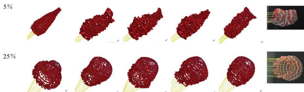
Figure 3. Change of the canopy shape during inflation ( t = 0.1, 0.3, 0.5, 0.7, 0.9 \text{ s} )
