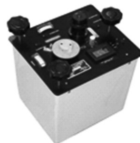
Fig. 5. LaCoste&Romberg model G gravimeter used for the collection of gravity data
