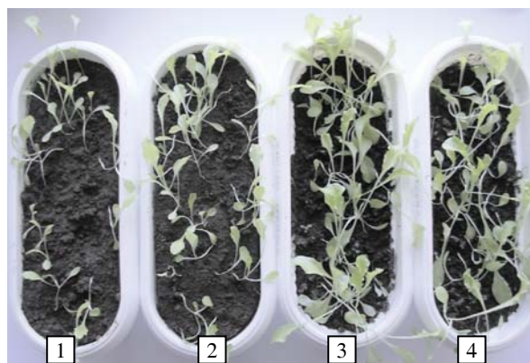
Fig 4. Lettuce samples were grown in substrates of different composition: 1, 2 – soil; 3, 4 – sewage sludge
