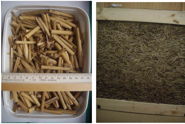
Fig. 5. Chopped reeds as the specimens of a random mix (thickness of 50 mm)
