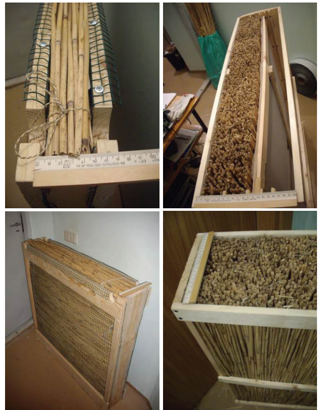
Fig. 2. The specimens of whole reeds are presented by four types of thickness
