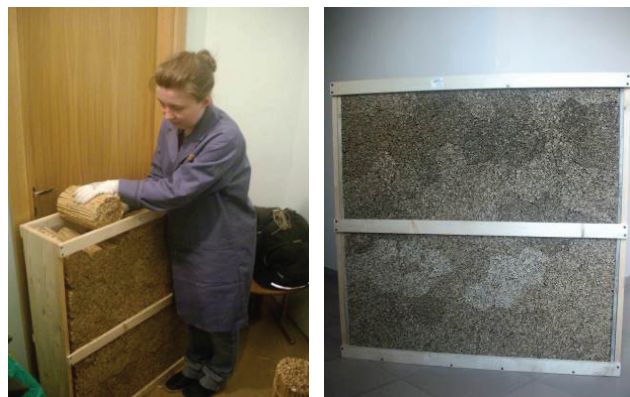
Fig. 3. The process of preparing the specimens of chopped reeds (200 mm thickness)
