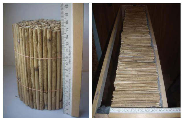
Fig. 4. The process of preparing the specimens of chopped reeds (150 mm thickness)
