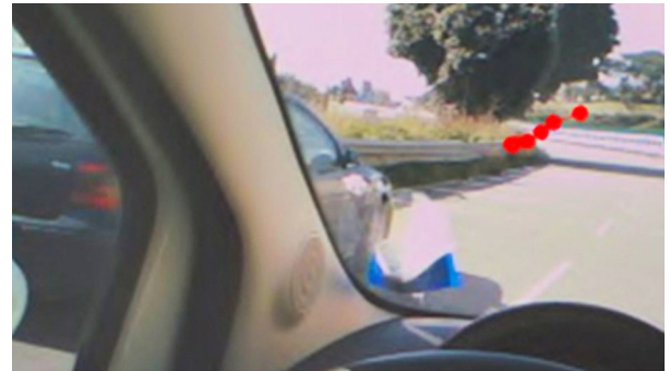
Fig. 7. Fixations are concentrated on the inner edge even if there is a passing vehicle
