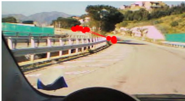
Fig. 5. The driver not only sets the tangent point of the curve but also the maximum sight distance. In this case, has tried to overcome the obstacle of the trees
