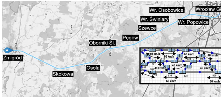
Figure 2. Simulated railway line with speed restrictions on switches near Wrocław Główny station (source: elaborated by the author using the OpenRailwayMap – https://www.openrailwaymap.org )
