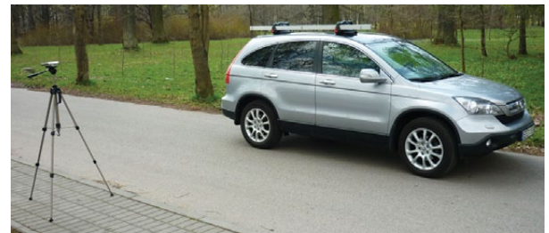
Fig. 3. System for precise velocity measurement with laser
